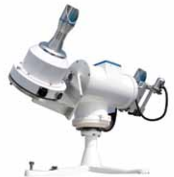
An MS-56 pyr heliometer and an MS-700 DNI sensor mounted on an STR-22G
