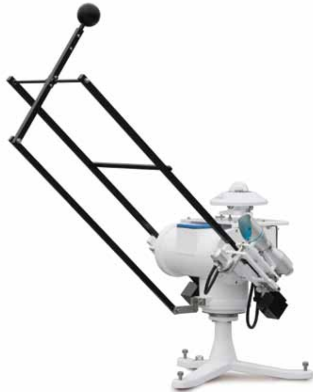
MS-802 pyranometer mounted on top of an STR-22G Sun tracker. The shading ball is used for the measurement of diffuse radiation.
