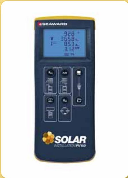
A variety of instruments are available for the PV installer, but it is important to make sure the correct instrument is selected and avoid products which only provide one or two tests, reducing the number of instruments needed as well as calibration requirements. The Seaward Solar PV150 is a hand held meter that performs a variety of tests in a safe and simple fashion.
